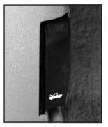
1. Pull the handle located inside the vehicle to the lower left of the steering wheel.
